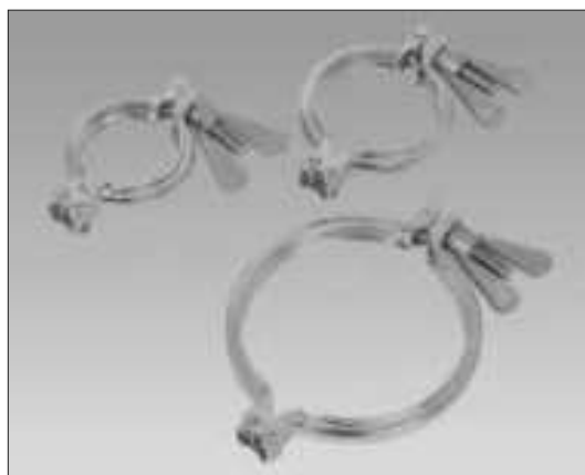
SP Type Clamp - Light Duty Sizes range from 1" through to 4", from DN25 through to DN100, Material AISI 304 stainless steel electropolished
